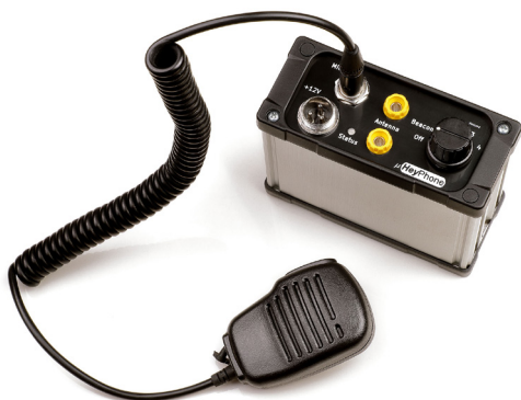
218. A \mu HeyPhone, the surface-mount rebuild of John Hey's original design. (Photo: Ian Cooper)
