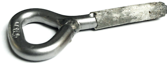
158. A glue-in anchor pulled out of a hole full of drilling dust. (Source: Deutscher Alpenverein e.V.: Bolts, 2nd edition, 2025)
